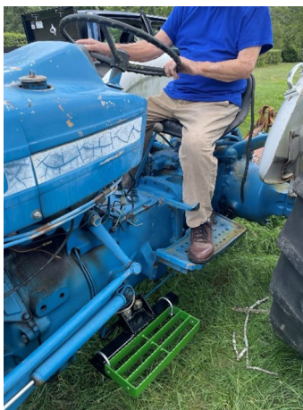
Green foot plate and small grab bar installed on the fender of a tractor to improve safety getting on and off farm equipment.
